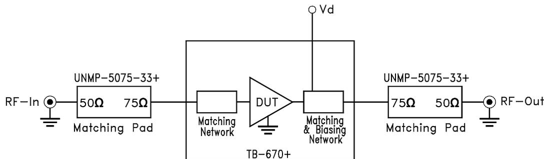
**Fig 1.** Block Diagram of Test Circuit used for characterization. (DUT tested on Mini-Circuits Characterization Eval board TB-670+) Gain, Return loss, Output power at 1dB compression (P1 dB), output IP3 (OIP3), output IP2 (OIP2) and noise figure measured using Agilent’s N5242A PNA-X microwave network analyzer.
